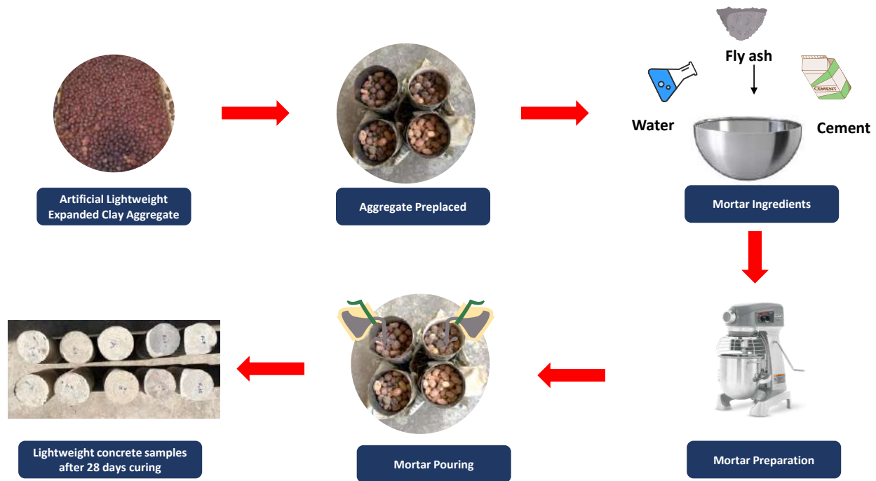
Fig. 26 Two stage casting process of lightweight concrete.
