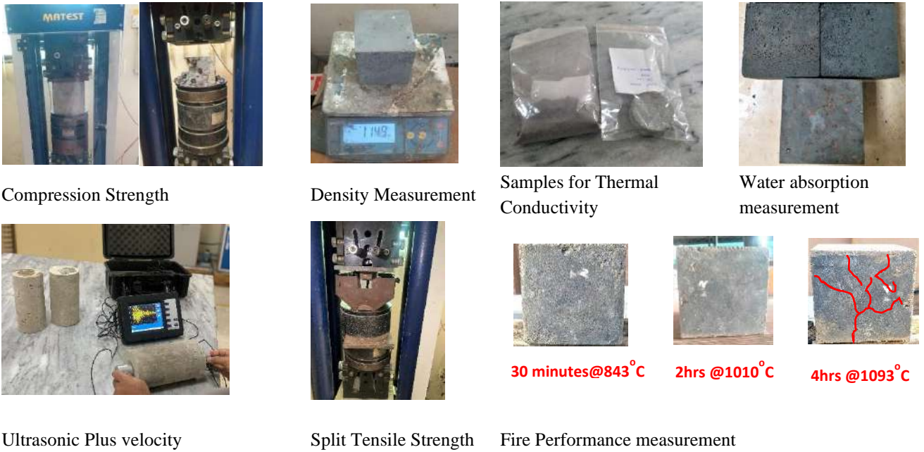
Fig. 27. Experimental program for performance assessment of ALECA infill lightweight concrete.
