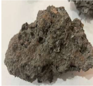
Figure 3-2 (a) Grit Scale Aggregates with rough and porous Structure
