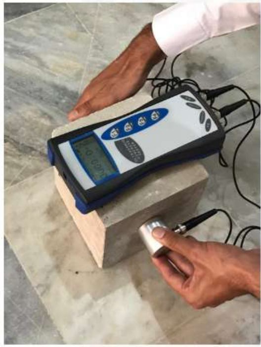
Figure 3-12 Ultra-sonic Pulse Velocity Test
