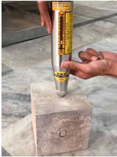
Figure 3-11 Rebound Hammer Test
