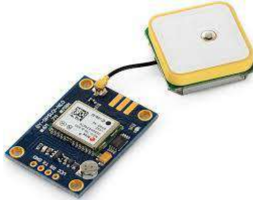
Figure 1.7 GPS module neo 6mv2
