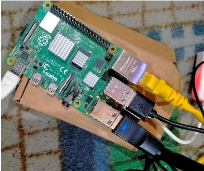
Figure 4 raspberry pi 4 interface connections
