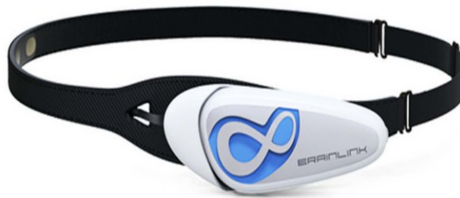
Figure 3.9: Brain Link Macro Tellec Device Used For Sensing Brainwaves [25]
