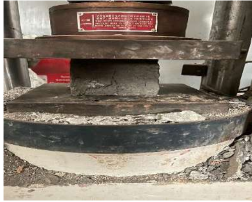
Figure 3 3 Compressive testing machine
