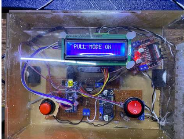
Figure 4.4: Arduino Nano paired with IBT-2 Module and voltage-current sensors in Control Box Unit during Pull Mode.
