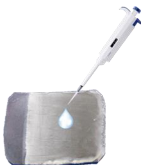
Fig 3.10. Contact angle measurement (wettability testing)
