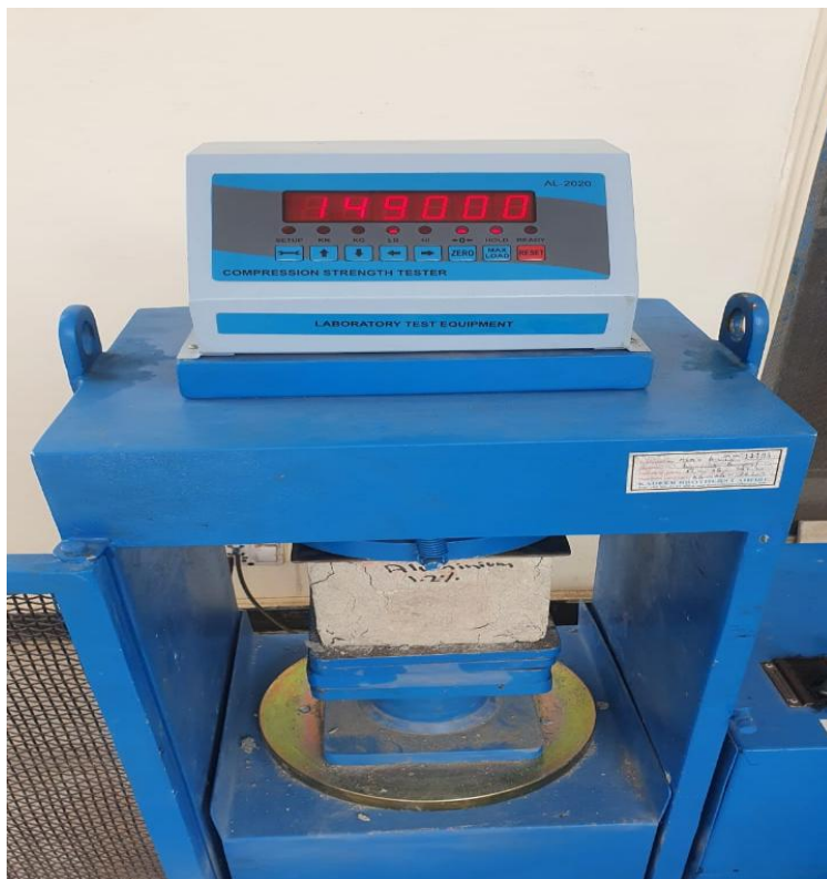
Figure 22: Compressive strength test (Aluminum Powder)-after applying load
