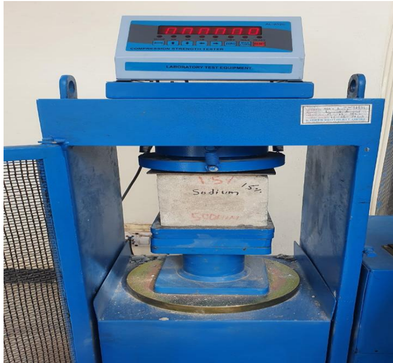
Figure 23: Compressive strength test (Sodium Carbonate)-Before applying load
