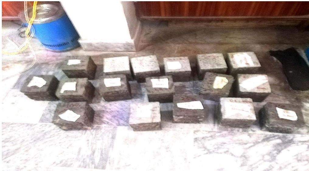
Figure 17: Samples removed from cube moulds after 24-hours
