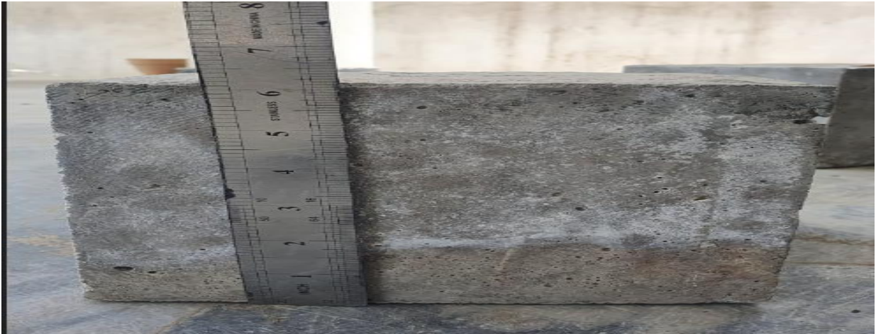
Figure 19: Measuring height of sample
