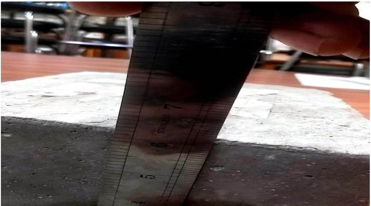
Figure 20: Measurement of height of different samples have admixtures (Change in the height observed)
