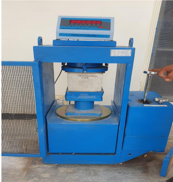
Figure 21: Compressive strength test (Aluminum Powder)-Before applying load
