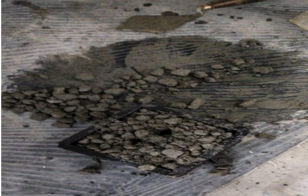
Figure 15: Pouring of mixture in cube mould
