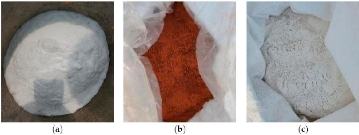
Figure 2. Types of additives. (a) High-polymer. (b) Red mud. (c) Metakaolin.
