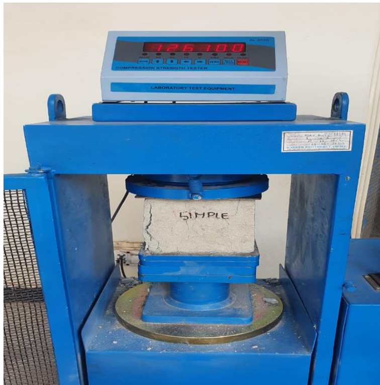
Figure 24: Compressive strength test (Sodium Carbonate)-After applying load
