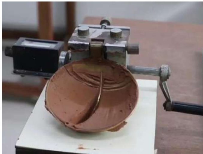
Figure 3.2. Determination of Liquid Limit Using Casagrande Cup Apparatus
