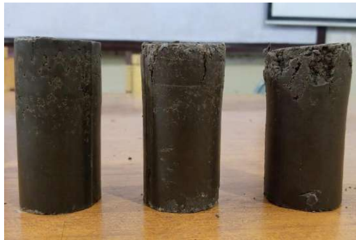
Figure 3.7. UU Test Sample Failure Planes
