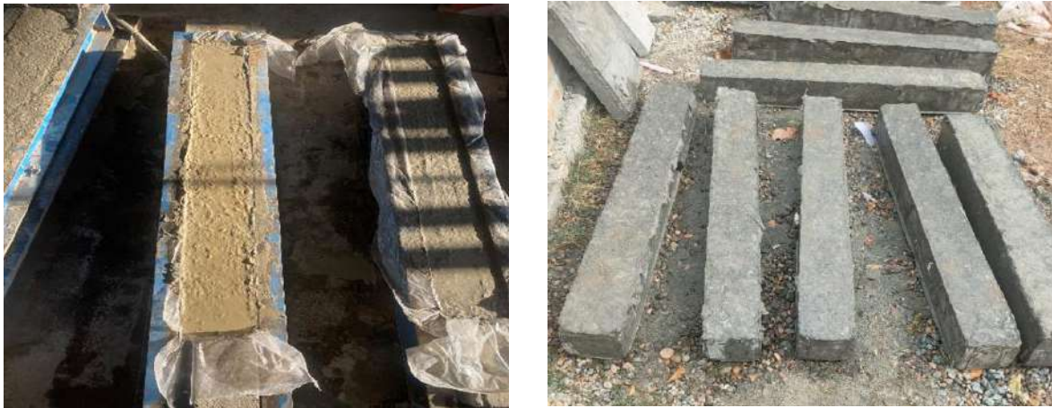
Figure 5.1 shows the casting of beams.
