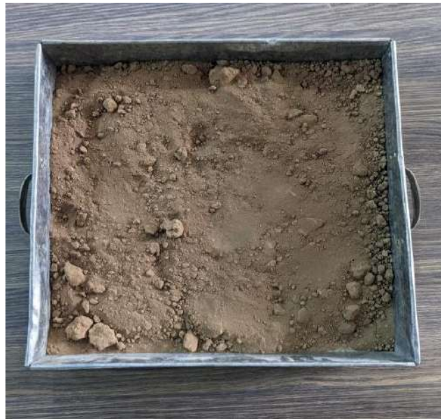
Figure 3.2. Oven dried natural soil sample.
