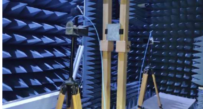
Fig 3.7 Electromagnetic interference shielding testing setup
