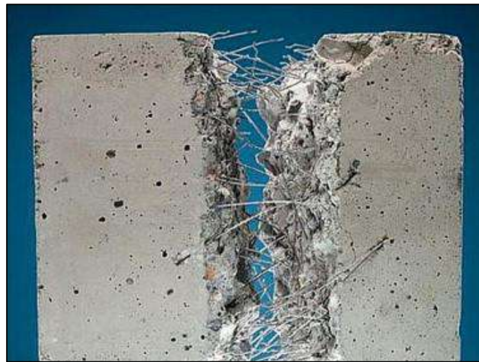
Fig 1.2 Crack arresting of steel fibers, reprinted with permission from Han, Baoguo Yu, Xun Ou, Jinping. Elsevier [5].
