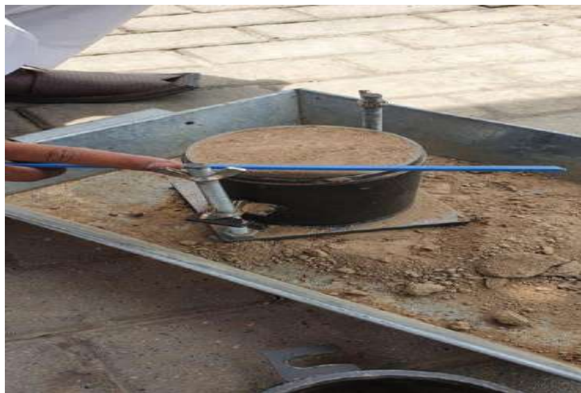
Figure 5 Cutting off extra soil from the mold with cutting edge
