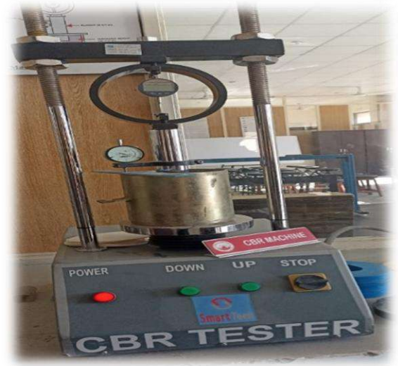
CBR test apparatus during testing
