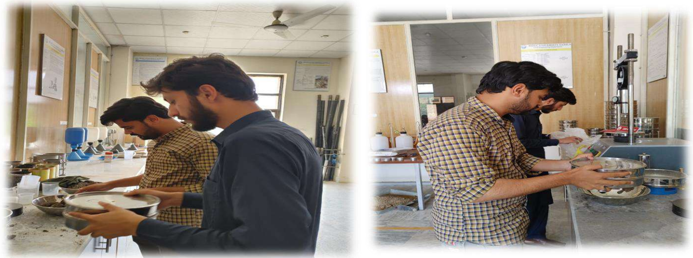
Figure 4 Sample preparation for Standard proctor Test
