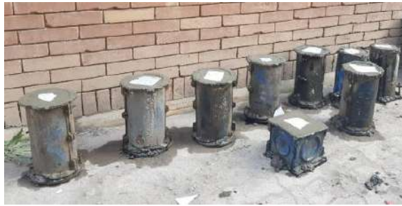
Figure 10: Casting of Samples
