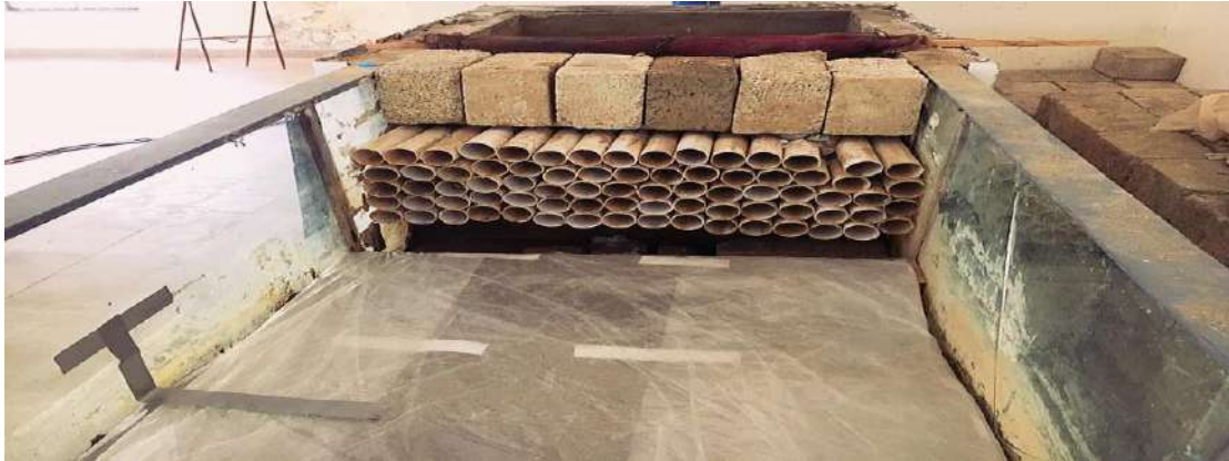
Figure 3.2: Straighter Pipes at the start of the channel
