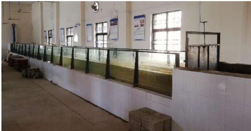
Figure3.1: Laboratory flume in Hydraulics Lab CED, UET
