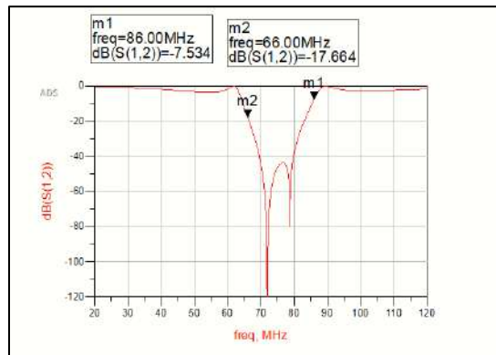
Figure 2.14: Simulation Results of IR Band-pass Filter
