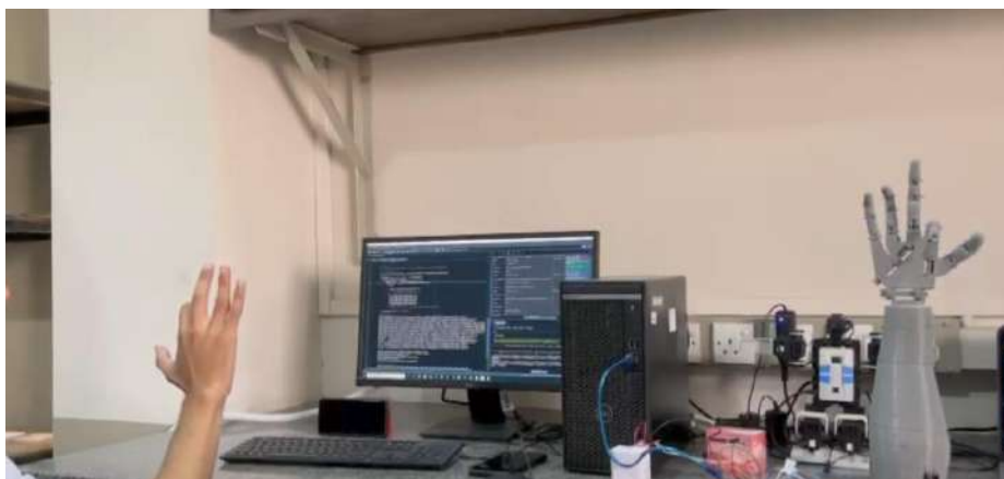
Figure 7.0.4 Index Finger testing [15]
