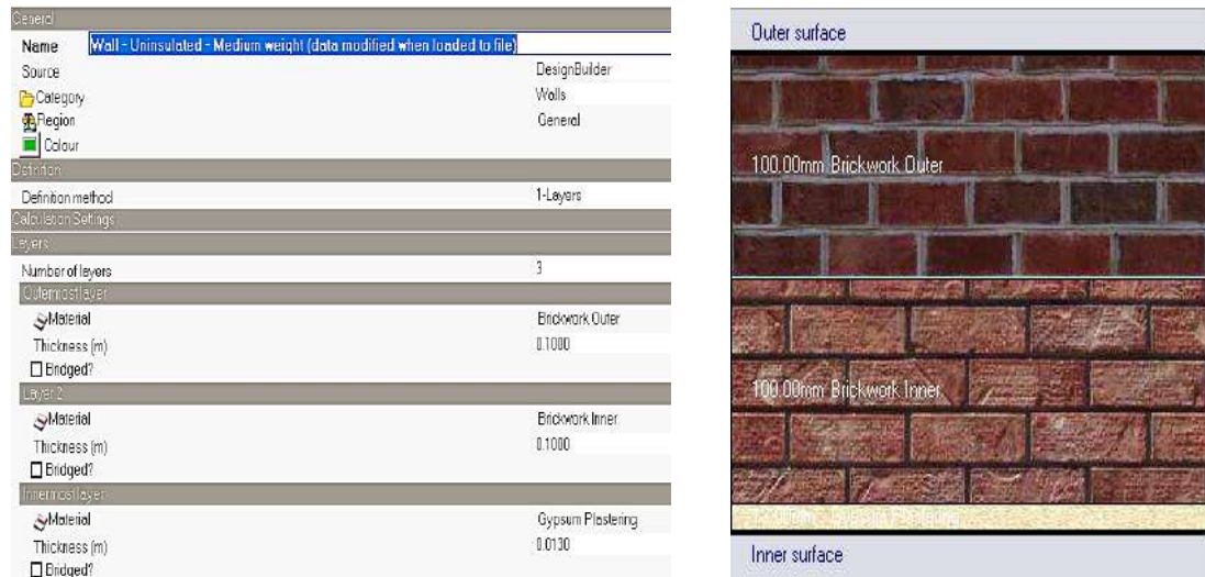
Figure 4.28: External wall construction in proposed building
