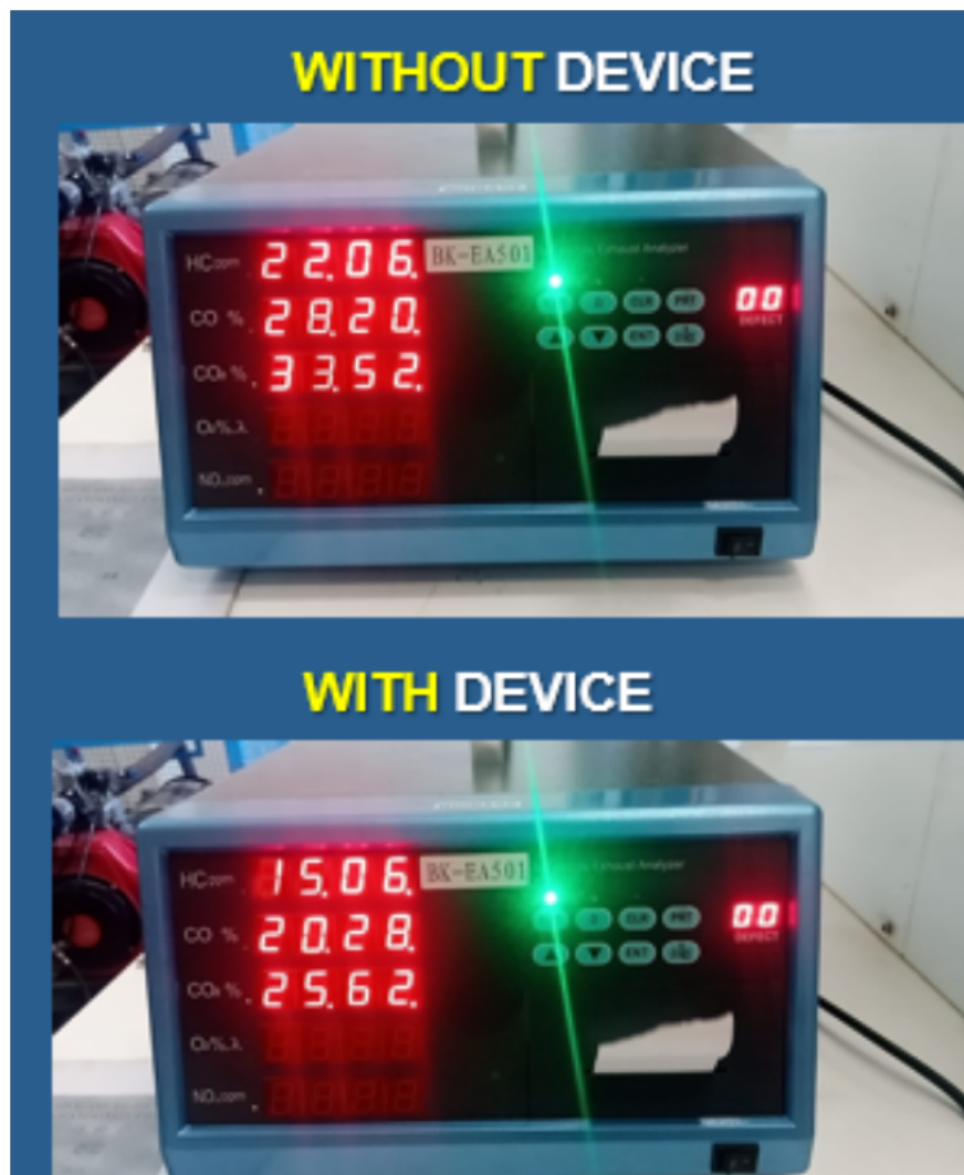
Figure 30: Results With & Without GREENV Device
