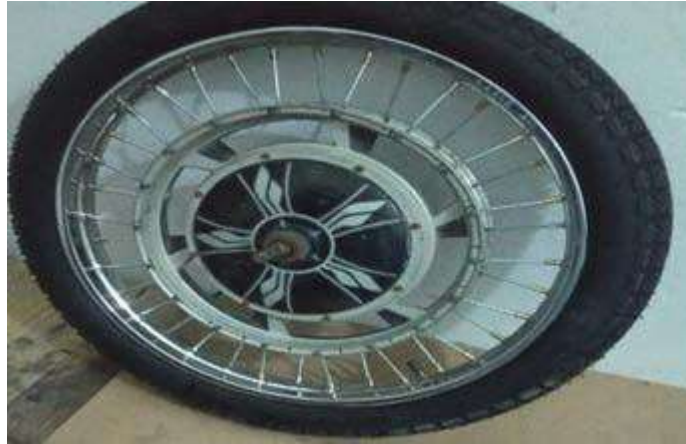
Figure 10 Tires with BLDC inside
