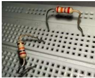
Fig 3: Voltage Divider Circuit
