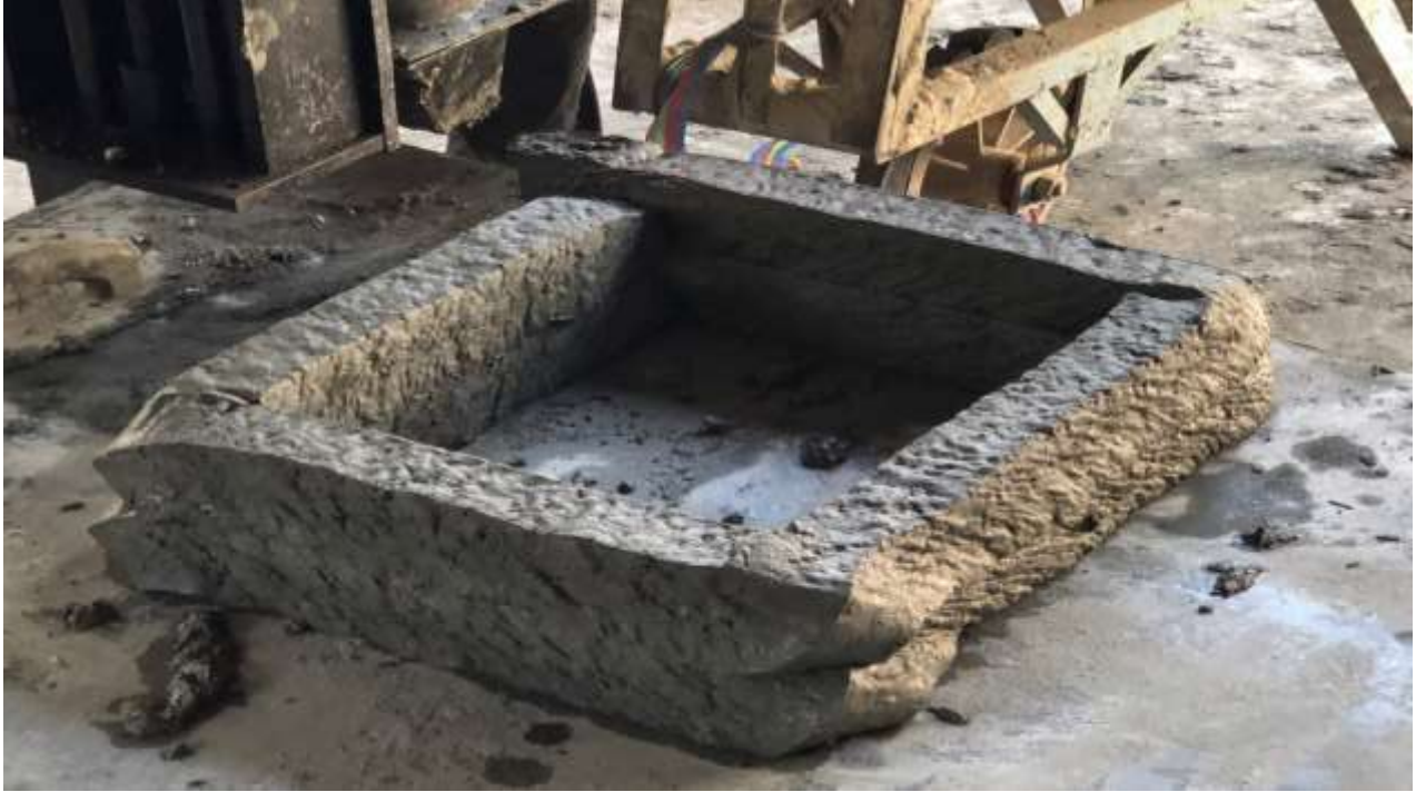
Figure 4.9: Printed Square with two layers upon each other.
