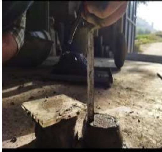
Figure 4.3: Deformation test under 500g loading.
