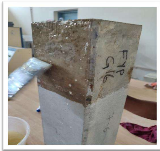
Figure 3.28 Applying of Epoxy
