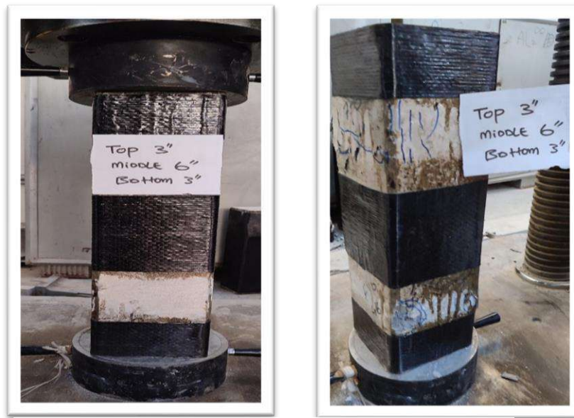
Figure 4.14 Before and After testing of T3", M6", B3"
