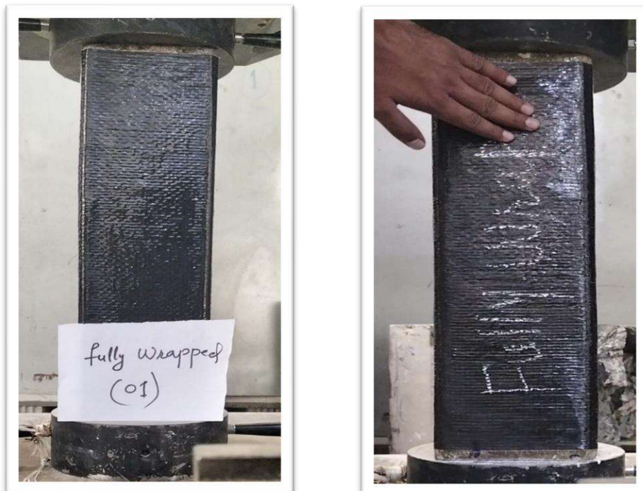
Figure 4.10 Before and After testing of fully wrapped
