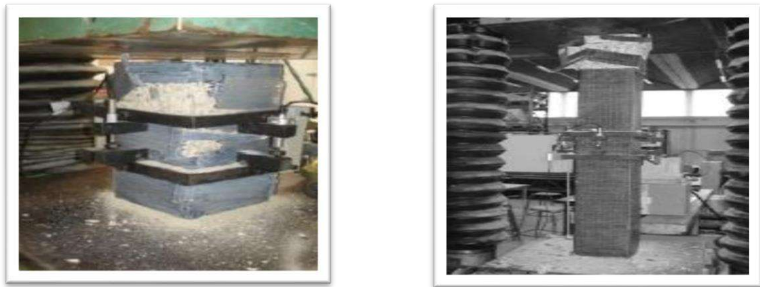
Figure 2.7 Confined CFRP Specimen Failure
