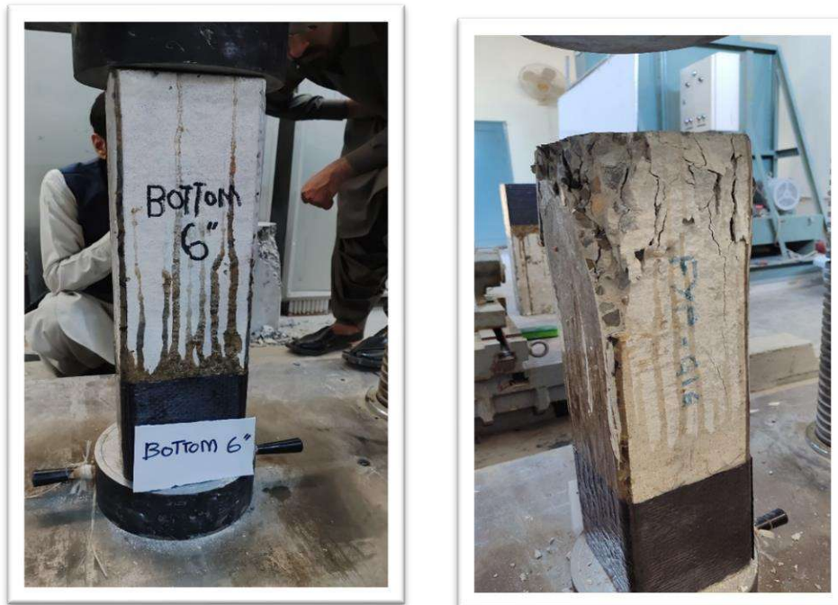
Figure 4.12 Before and After testing of bottom 6"
