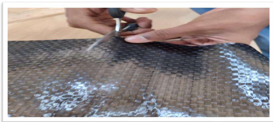
Figure 3.26 Cutting of CFRP sheets
