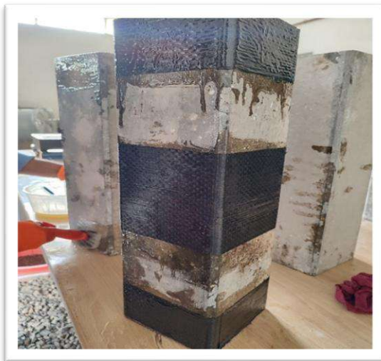
Figure 3.29 Wrapping of CFRP sheets
