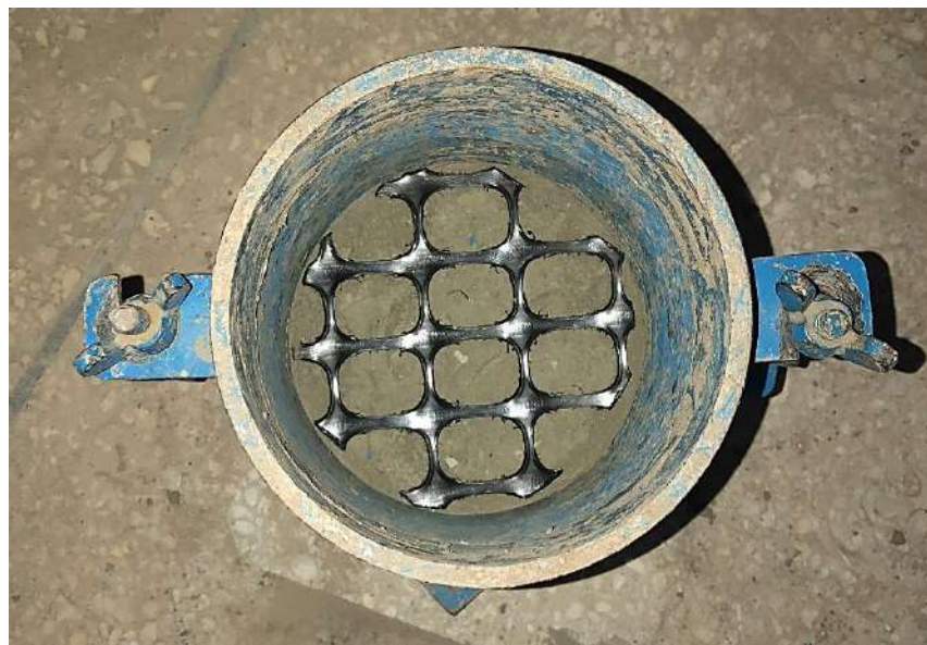
Figure 4.12: Shows Placing of Biaxial Geogrid in CBR mold
