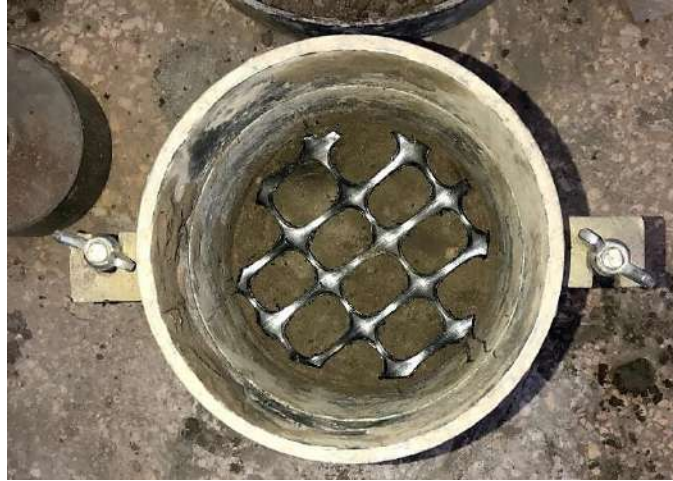
Figure 3.14: Placing Biaxial Geogrid in CBR mold
