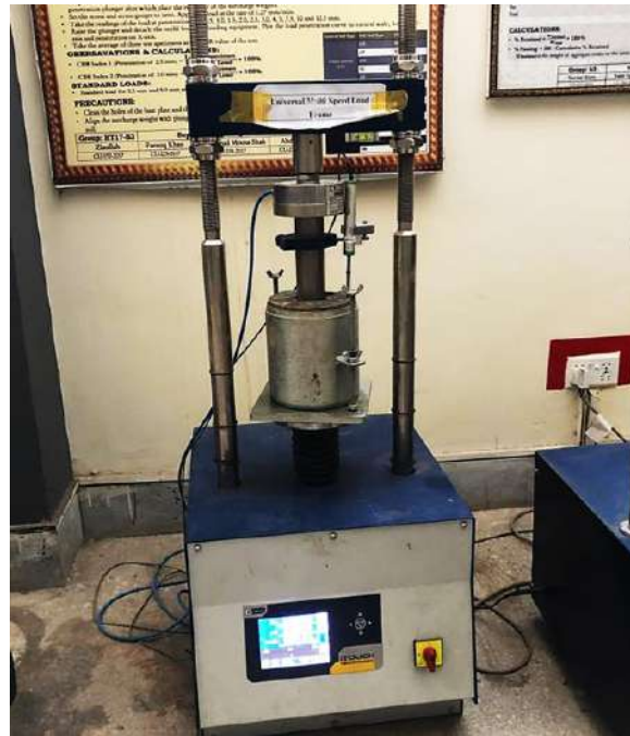
Figure 3.12: CBR (California Bearing Ratio) Test
