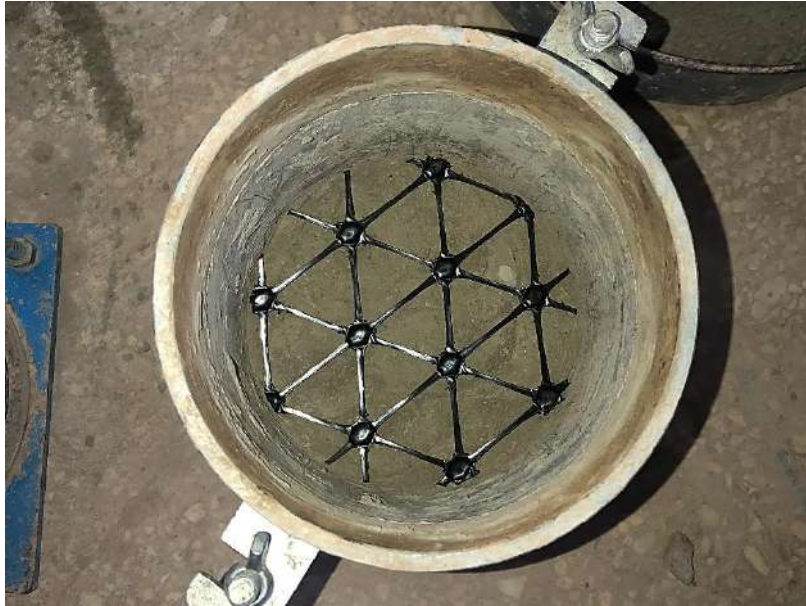
Figure 4.14: Shows Placing of Triaxial Geogrid in CBR mold
