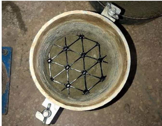
Figure 3.15: Placing Triaxial Geogrid in CBR mold
