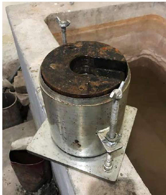
Figure 3.13: Placing CBR Mould in Water
