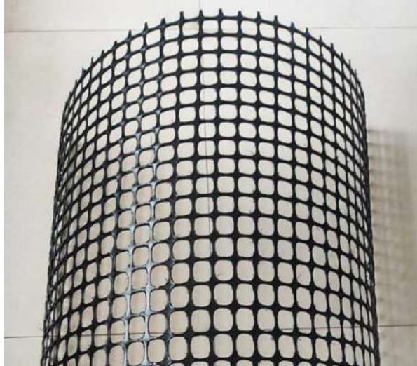
Figure 3.6: Geosynthetic Material (Biaxial Geogrid) used in this project
