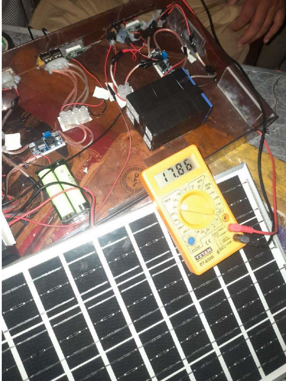
Figure 5.3: Boost converter testing
