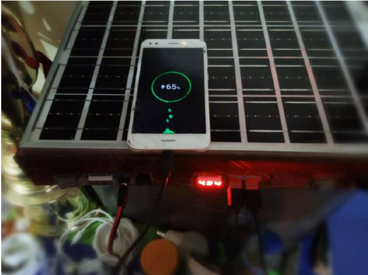
Figure 5.2: Buck converter testing
