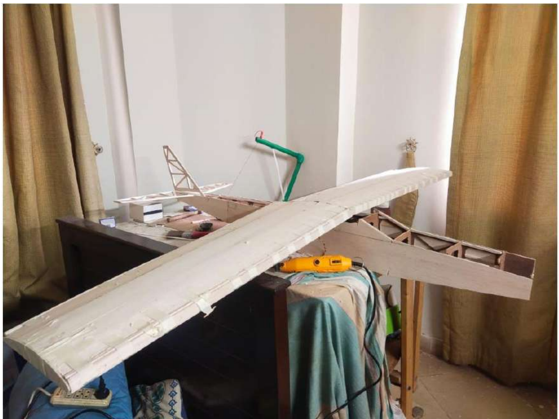
Figure 53: Assembled Fuselage, Tail and Wing
