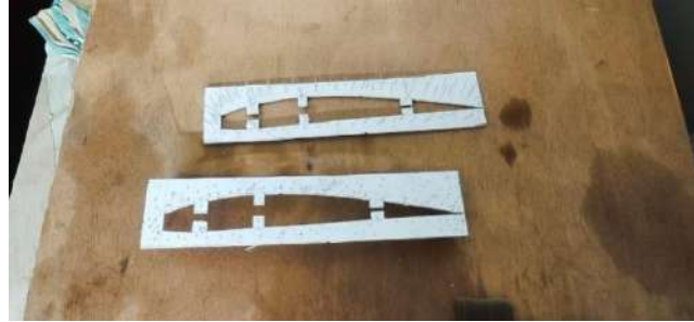
Figure 50: Cutting Out Airfoils Using the Template
