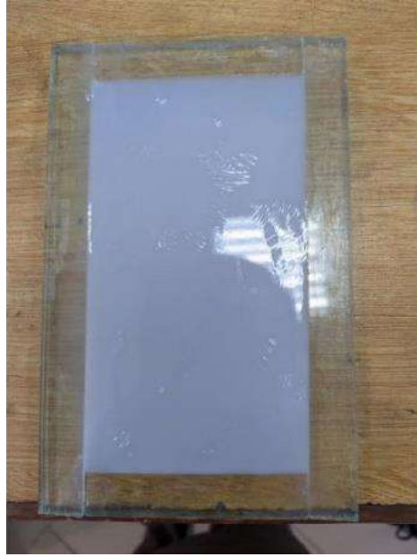
Figure 15: Casting into mold
