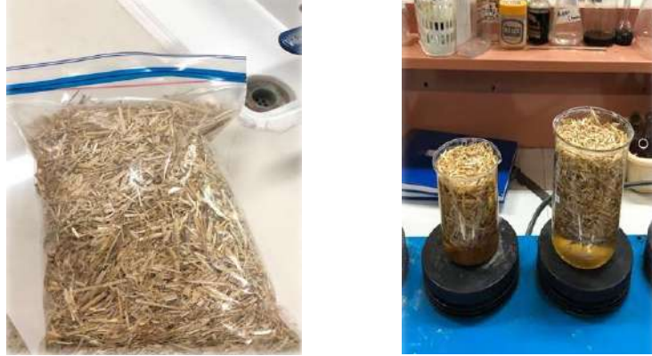
Figure 7: Sterilization using boiler method
