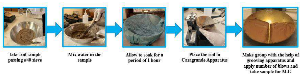
Figure 3.9: Liquid limit test Procedure
