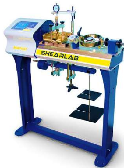
Figure 3. 12: Direct Shear test apparatus used for experiment
