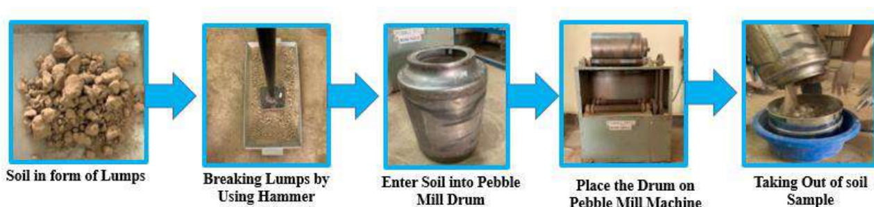
Figure 3.4: Pulverization of soil using Pebble Mill Apparatus
