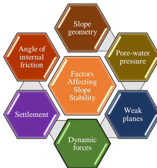
Figure 2.19: Factors effecting stability of slopes
