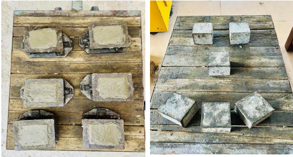
Figure 4.13: Casting of Cubes for Concrete Compressive Strength
