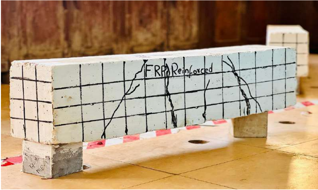
Figure 4. 22: Cracks Pattern in FRP Beam 3
