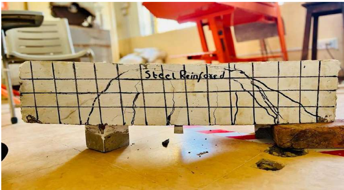
Figure.4. 17: Cracks Pattern in Steel Beam 1
