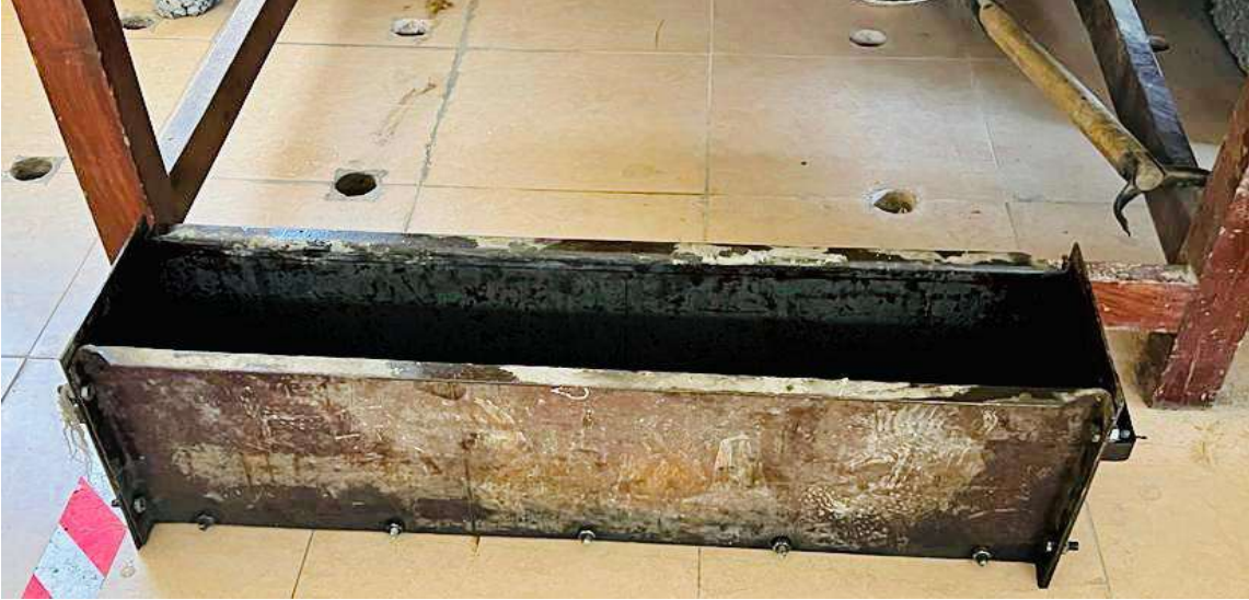
Figure:4.7: Mould of Steel and FRP Beam.
