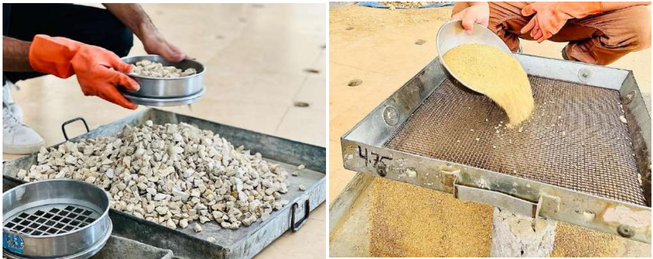
Figure 4.6: Sieve of fine and coarse aggregates
