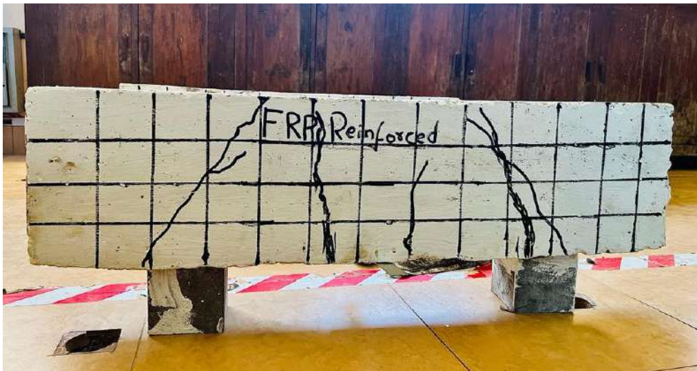
Figure 4. 21: Cracks Pattern in FRP Beam 2
