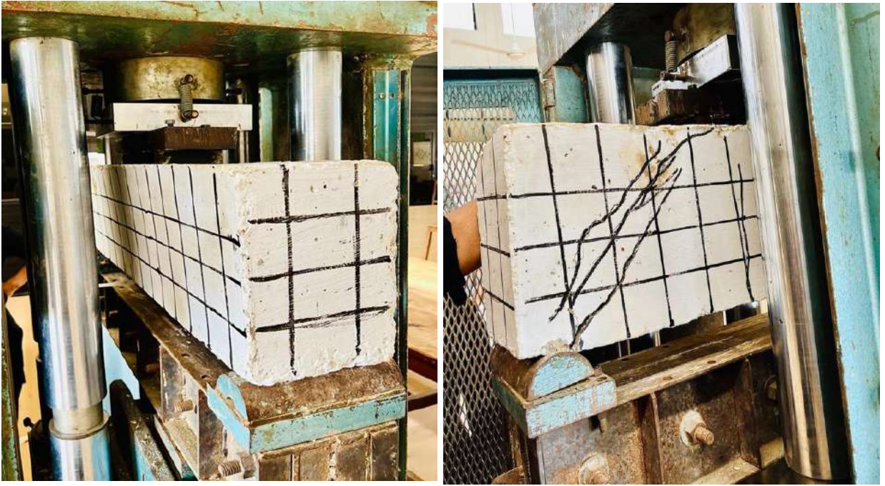
Figure.4. 16b: Four Point Beam testing in UTM
