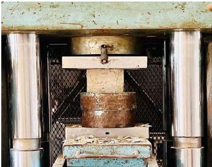
Figure 4.14a: Testing of cubes
