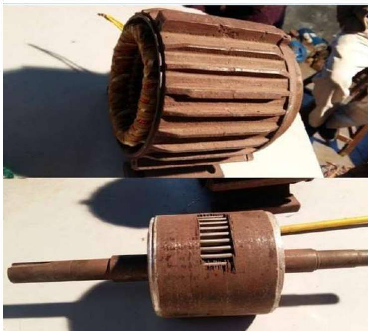
Fig.2.7: Healthy stator but Unhealthy rotor (rotor core problem)
