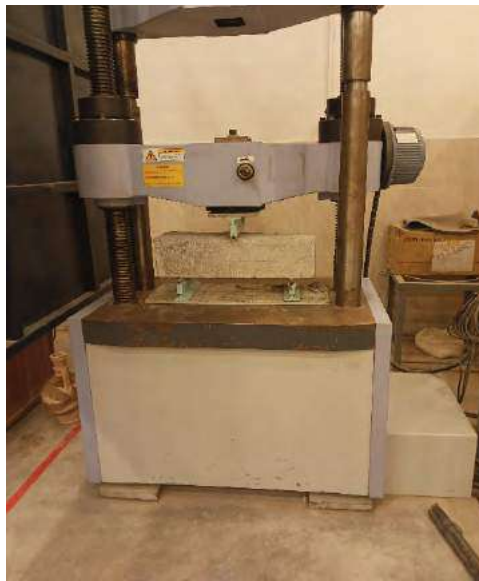
Figure 3.22: Flexural strength test center point loading
