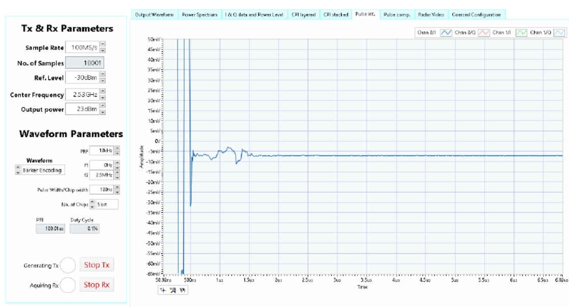
Figure 5-13: Pulse Integration for 5-Bit Barker
