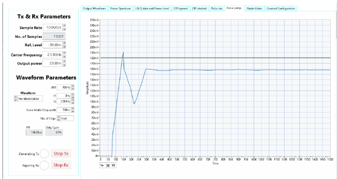
Figure 5-20: Matched Filtering of Basic Pulse
