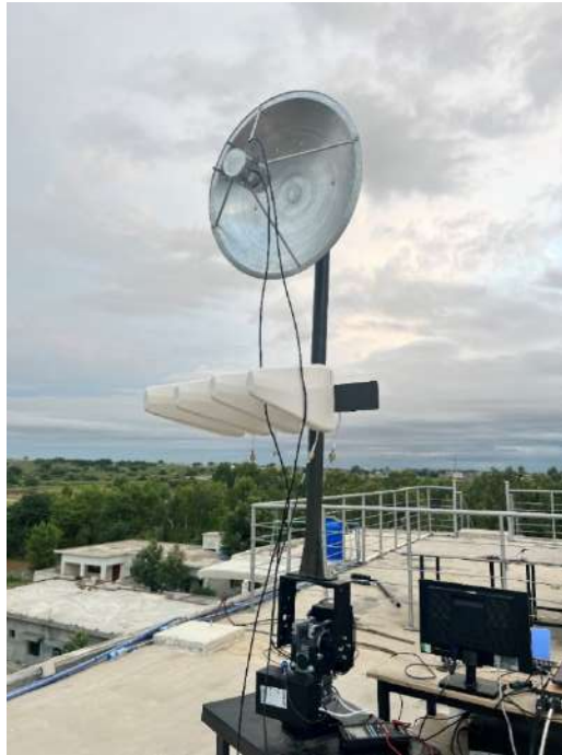
Figure 3-21: Tx and Rx Antennas Mounted on A Rotator for Radar
