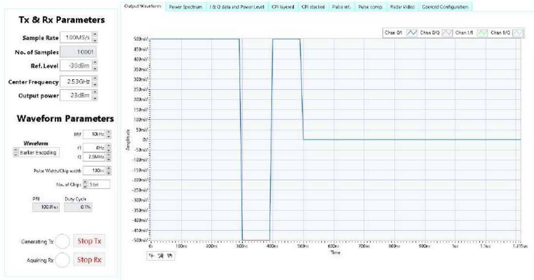
Figure 5-10: Barker Encoding 5-Bit Transmission Pulse
