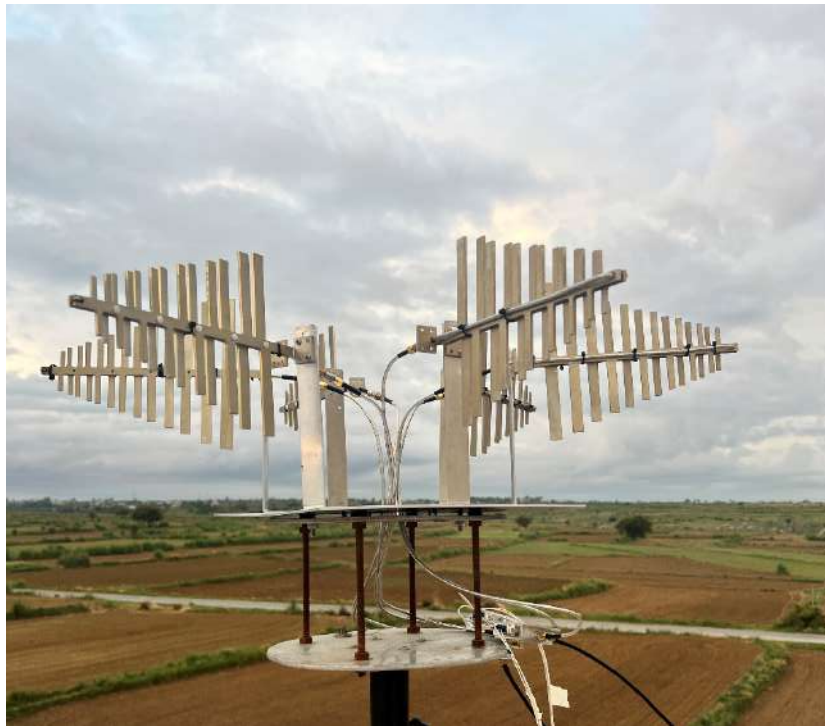
Figure 3-20: 6 Element Switched Array For DF
