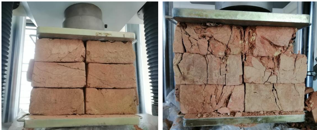
Figure 3.10 Interlock Brick Sample Before and After Prism Test
