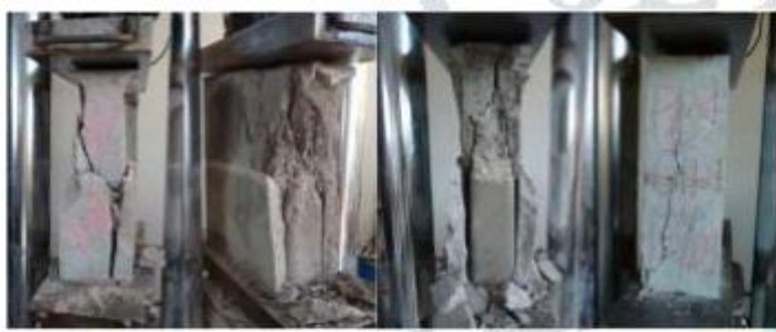
Figure 2.6 Samples during compressive strength test
