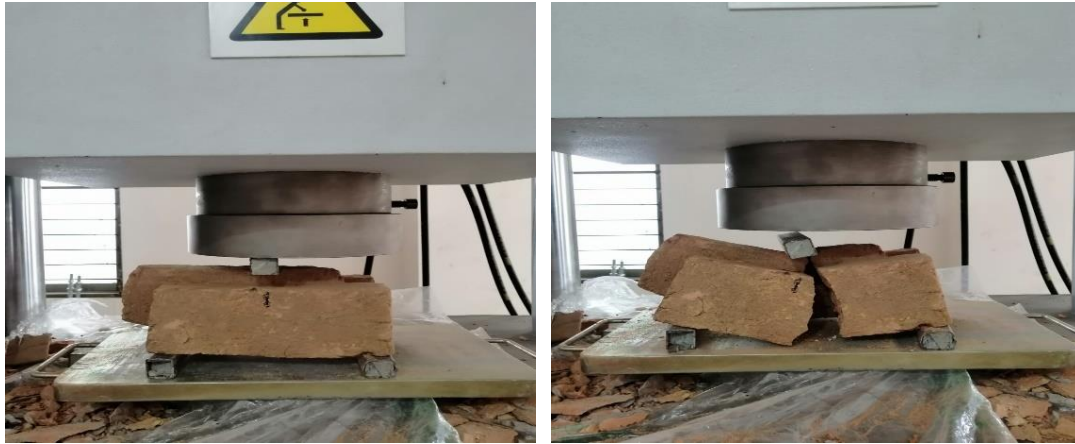
Figure 3.9 Test Samples Before and After Flexural Failure
