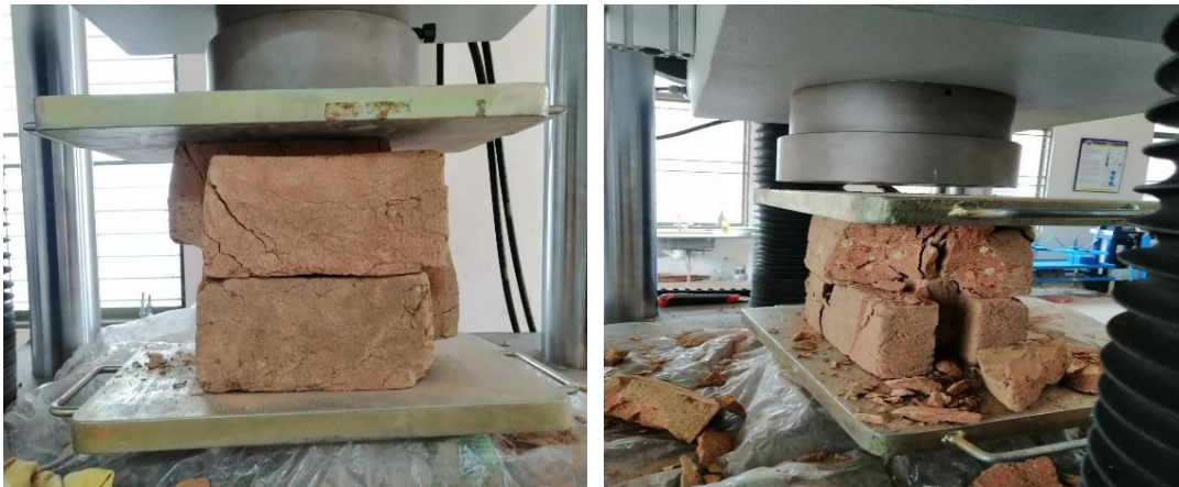
Figure 3.7 Double Brick Sample Before and After Test
