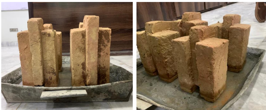
Figure 3.11 Samples for Efflorescence Test
