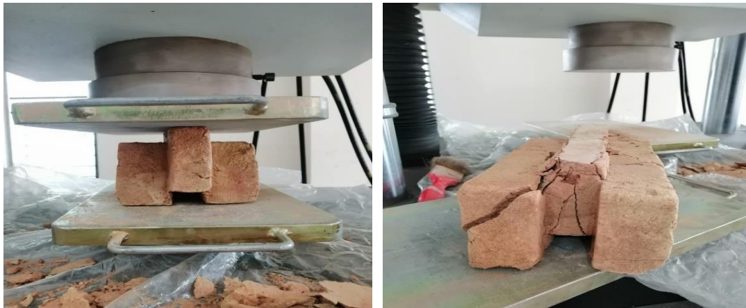
Figure 3.4 Interlock Brick Sample Before and After Test
