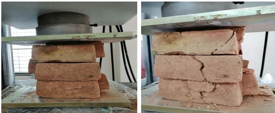
Figure 3.8 Double Brick Sample Before and After Test
