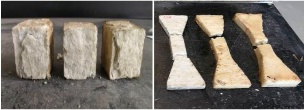
Figure 2.8 Samples after compressive and split tensile strength test
