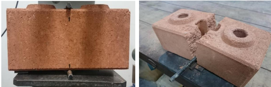
Figure 2.7 Interlock brick during flexural strength test
