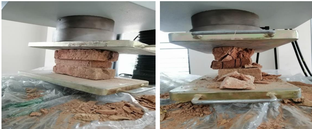
Figure 3.5 Side Wise Sample of Interlock Brick Before and After Test
