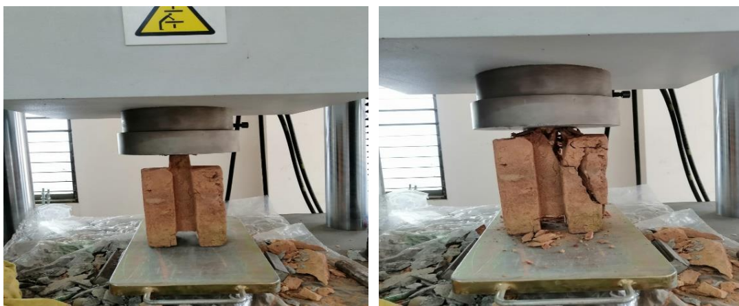
Figure 3.6 Vertical Sample of Interlock Brick Before and After Test
