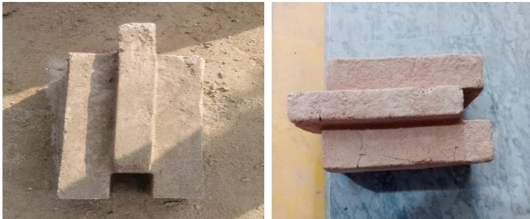
Figure 3.2 Samples of interlock bricks before and after heating in kiln
