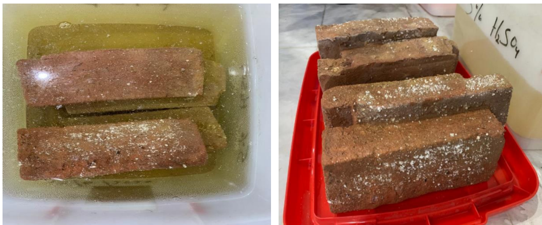
Figure 3.13 H 2 SO 4 Immersed Interlock Bricks
