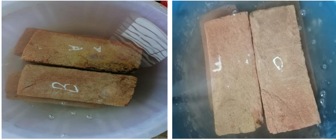
Figure 3.3 Interlock bricks sample when immersed in water
