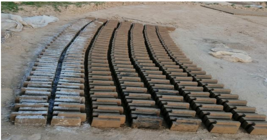
Figure 3.1 Manufacturing of interlock bricks
