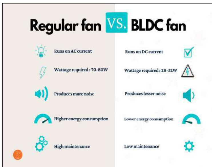
Figure 4.54: Comparison of BLDC fan with a regular fan ( CAG )
