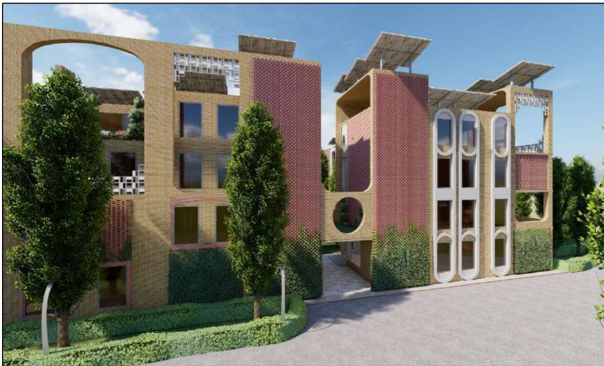
Figure 4.40: 3D view showing walls with thermal mass bricks and creeper plants
