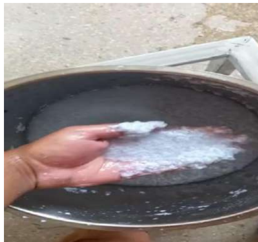
Figure 4.5: Repulp of waste paper
