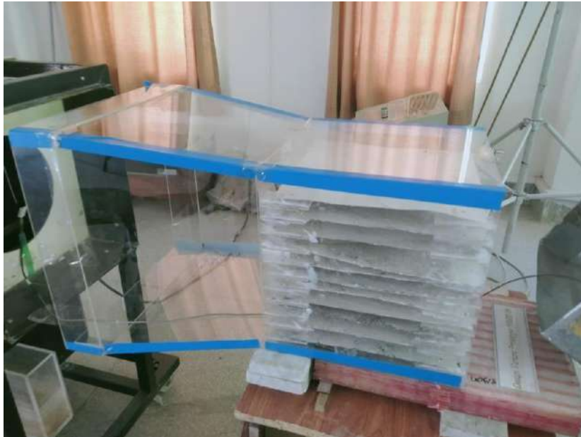
Figure 4.41: Ducts with Coated Aluminium Sheets
