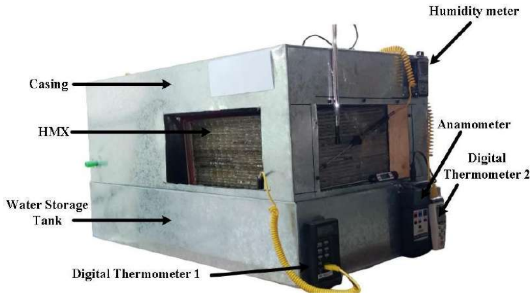
Figure 4.22: The experimental setup of design variant prototype 06 with measuring sensors (External view)
