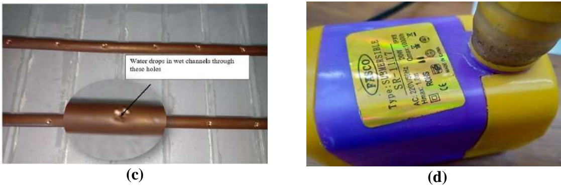
Figure 4.2: Different fabrication phases (a) holes creation in the dry channel, (b) zig zag holes pattern, (c) copper pipes with holes for water flow, (d) pump used for pumping the water in the wet channels
