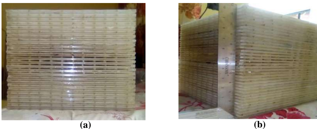
Figure 4.12: Different views of the HMX of DVP 04 (a) working air side view, (b) symmetric view
