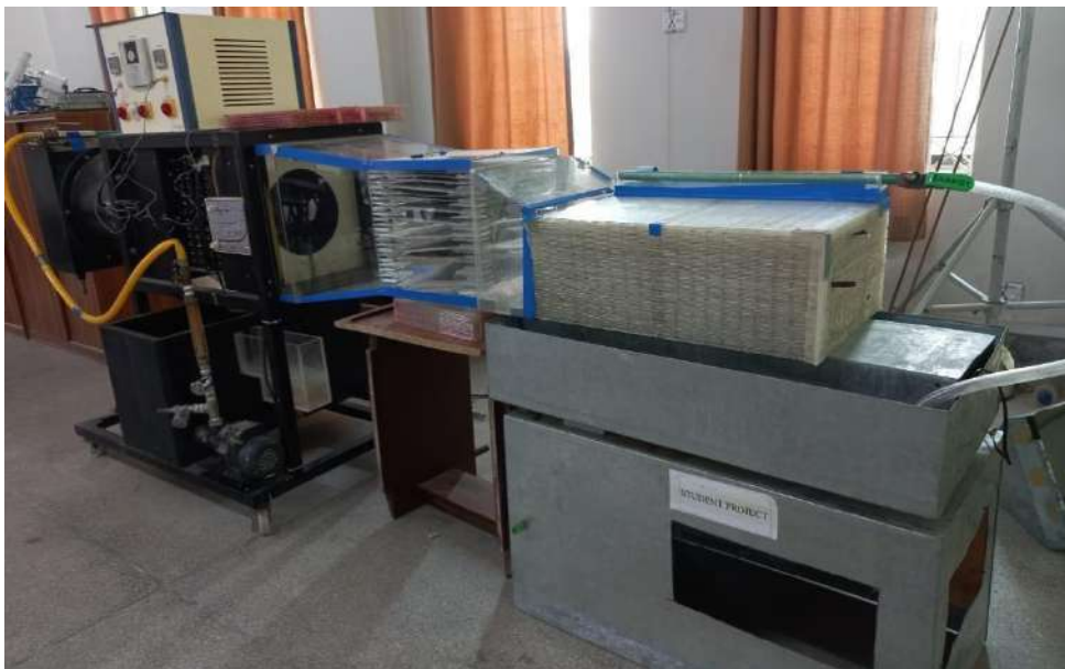
Figure 4.47: Experimental Setup of HMX with Dehumidification Bed
