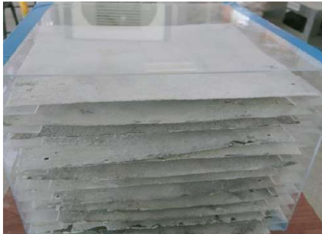
Figure 4.42: Silica Gel Coating on Aluminium Sheets
