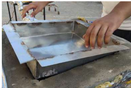
Figure 4.16. Placing Boiling Pan on Furnace
