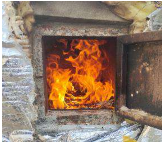
Figure 4.19. Burning of Bagasse in Furnace
