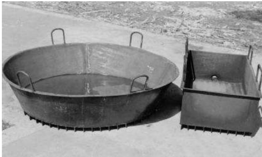
Figure 2.7. Modified traditional main pan and gutter pan.
