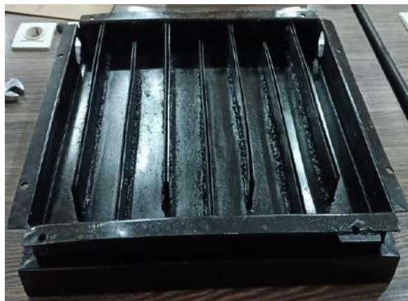
Figure 4.9 Fabricated Pre Heated Exhaust Chamber
