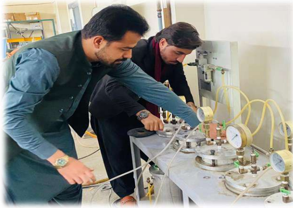
Figure 5-6 water permeability test
