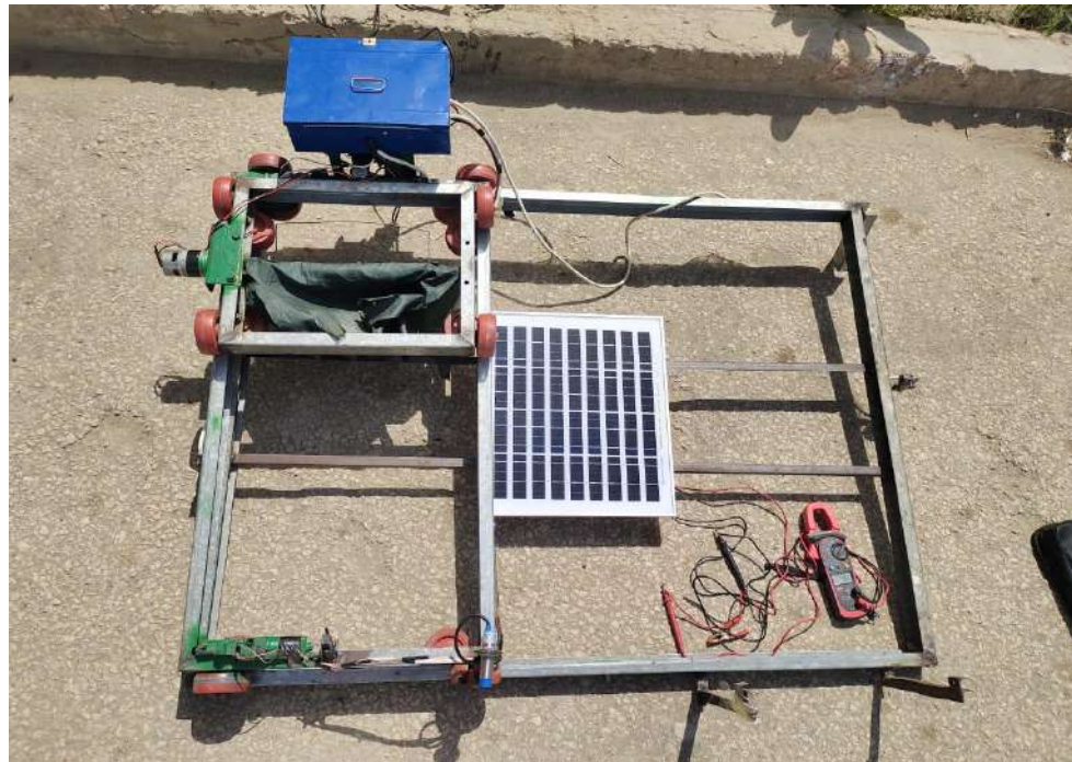
Figure 26: Solar panel's voltage after cleaning.
