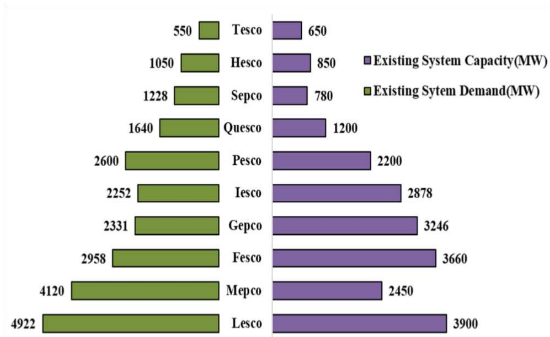
Figure 1: Comparison of system capacity and energy demand for different suppliers in Pakistan [1].
