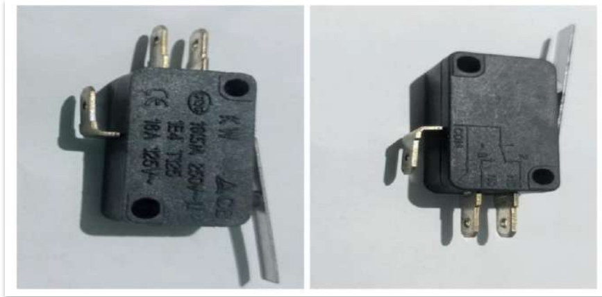
Figure 15: Limit Switch [@ control lab]
