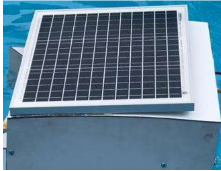
Figure 3.15: Solar panel mounted on lake/pool cleaner drone
