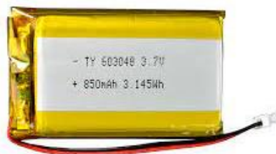
Figure 8 Lithium Ion battery
