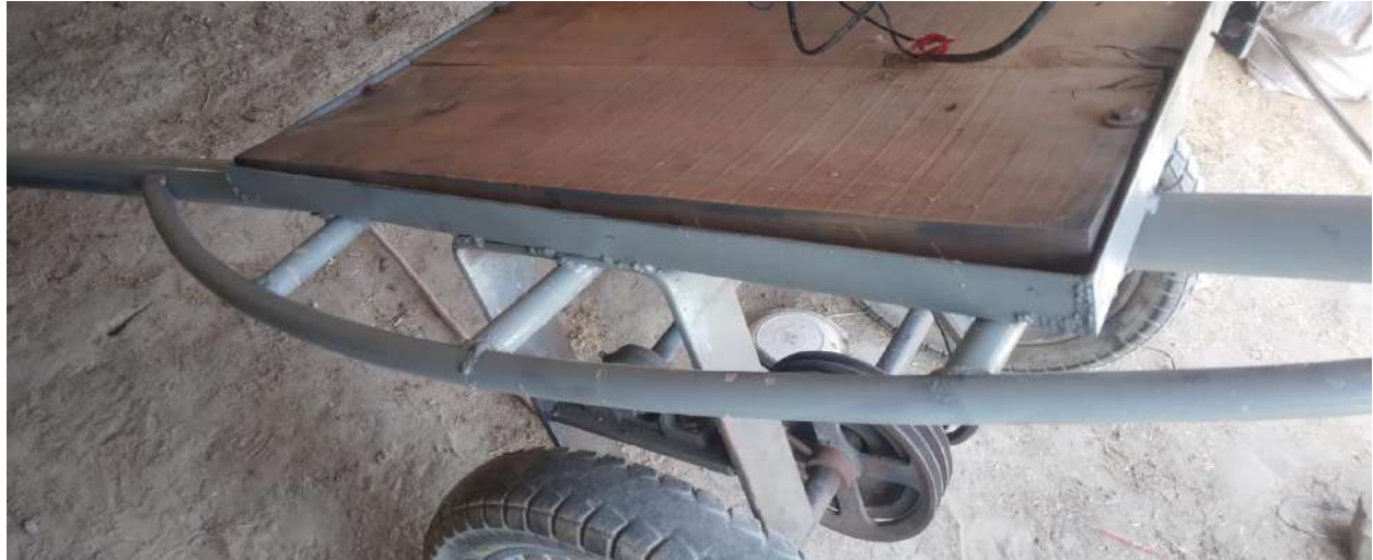
Fig 4.24: Iron pipe in curved form [11-04-23]
