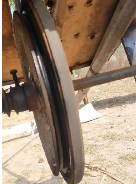
Figure 4.3: Pulleys (14 & 16 inches) on 2 nd axle [25-01-23]
