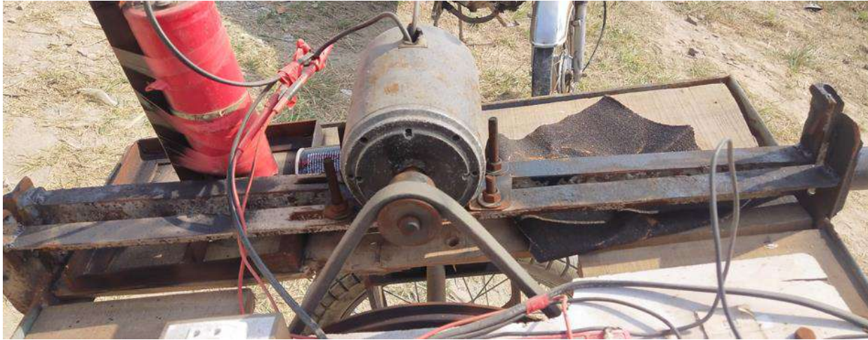
Figure 4.7: Support for generator [05-02-23]
