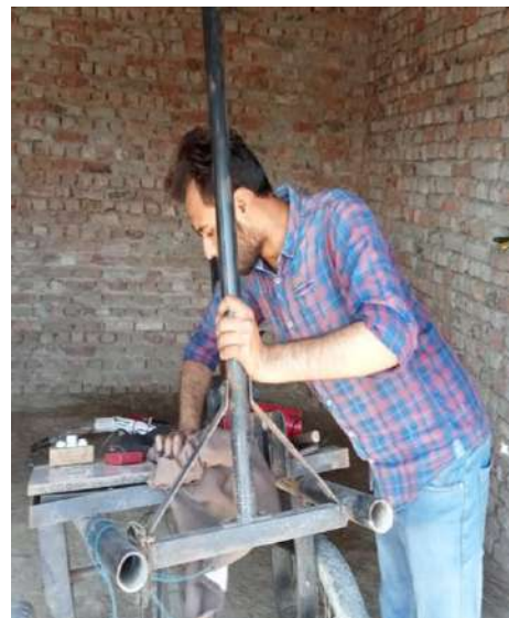
Figure 4.17: cleaning of rust by sandpaper [08-03-23]
