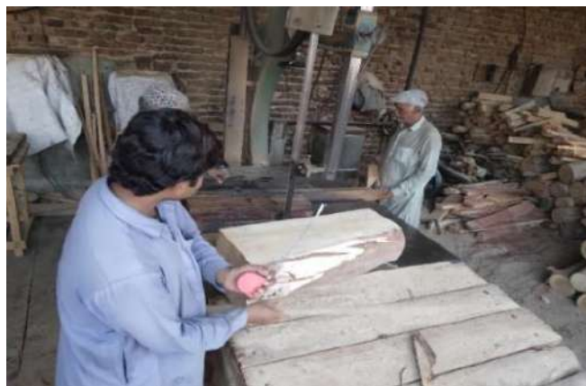
Figure 3-18: Cutting of wooden boards [11-10-22]
