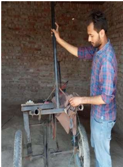
Figure 4.16: cleaning of rust by sandpaper [08-03-23]
