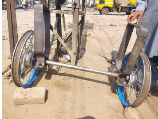
Figure 3-11: Cart (wheels, axle, support) [27-9-22]
