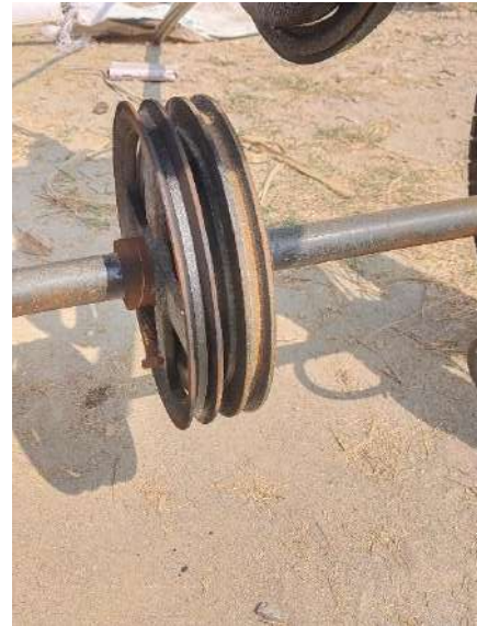
Figure 4.2: Pulleys (10 inches) on 1 st axle
