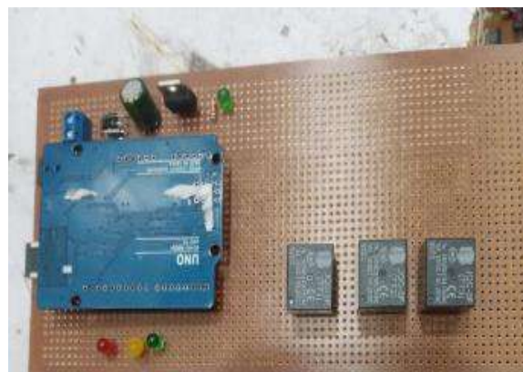
Fig no. 5.9: Assembling of relays with Arduino Uno 08-03-2023
