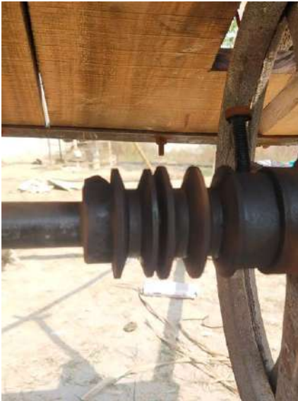
Figure 4.1: Pulleys (2.5 inches) on 2 nd axle [21-01-23]
