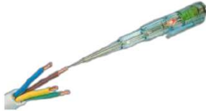
Figure 61: Detection of live wire using tester.
