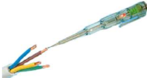
Figure 61: Detection of live wire using tester.
