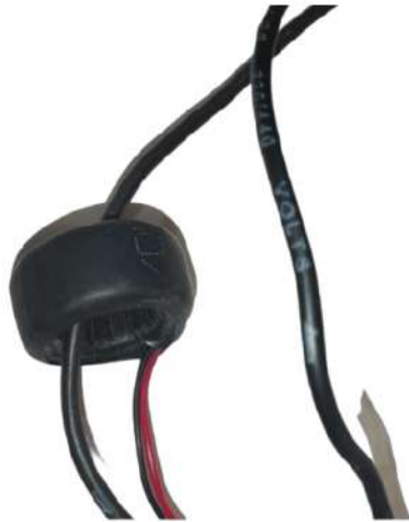
Figure 63: Live Wire Through CT connected to Load.
