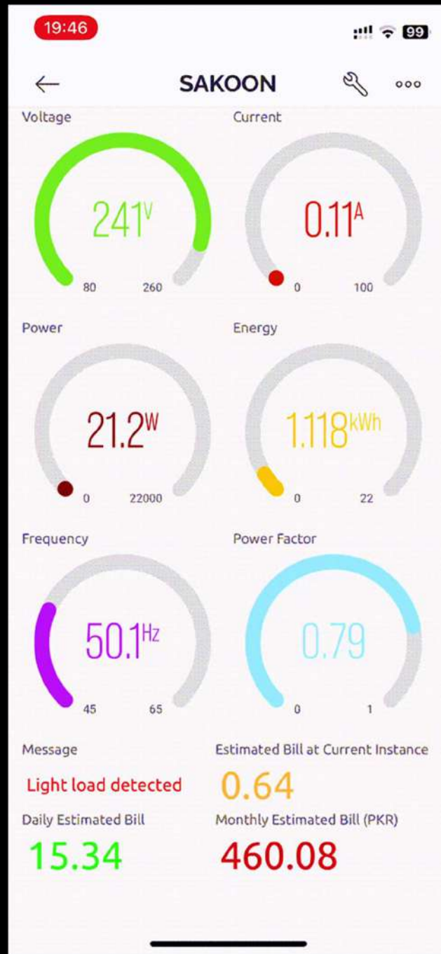
Figure 21: Mobile App showing real time energy consumption and estimated bill.
