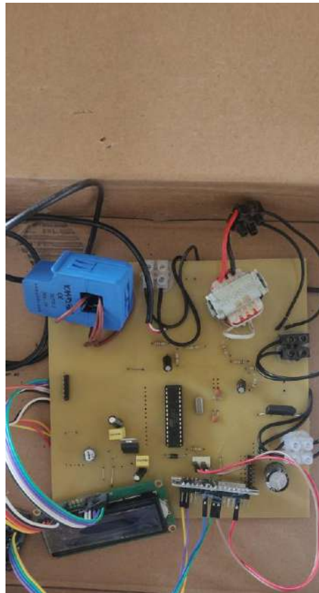
Figure 4.19: Energy meter hardware
