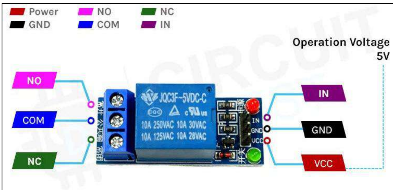
Figure 4.10: Relay Module Pin-out [18]
