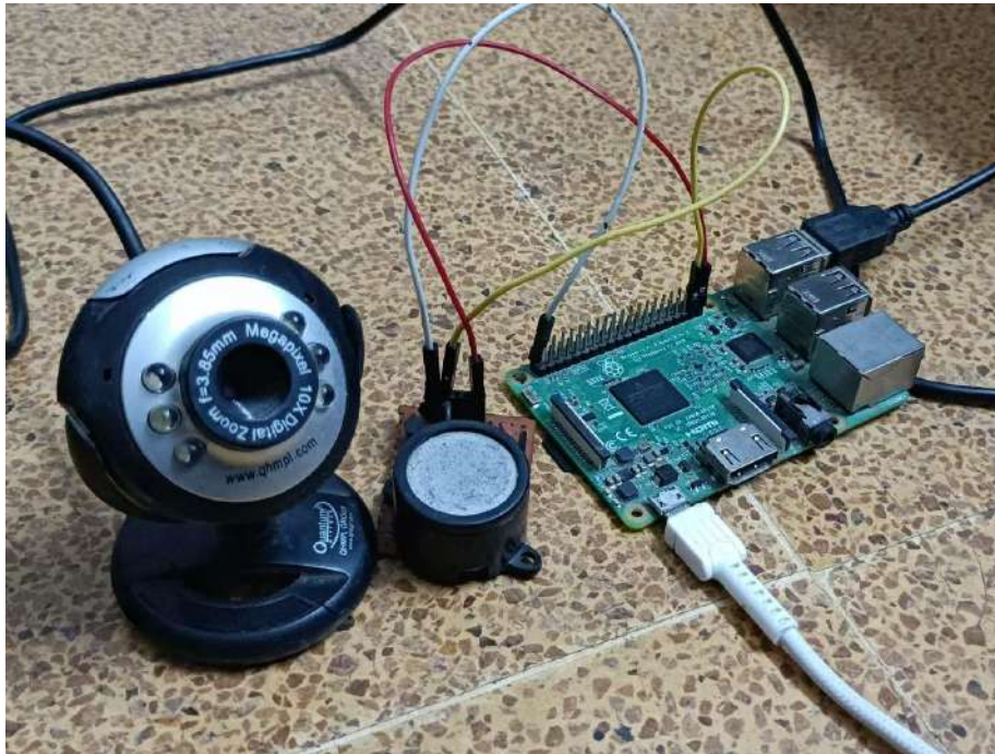
Figure 4.3: Camera for drowsiness detection
