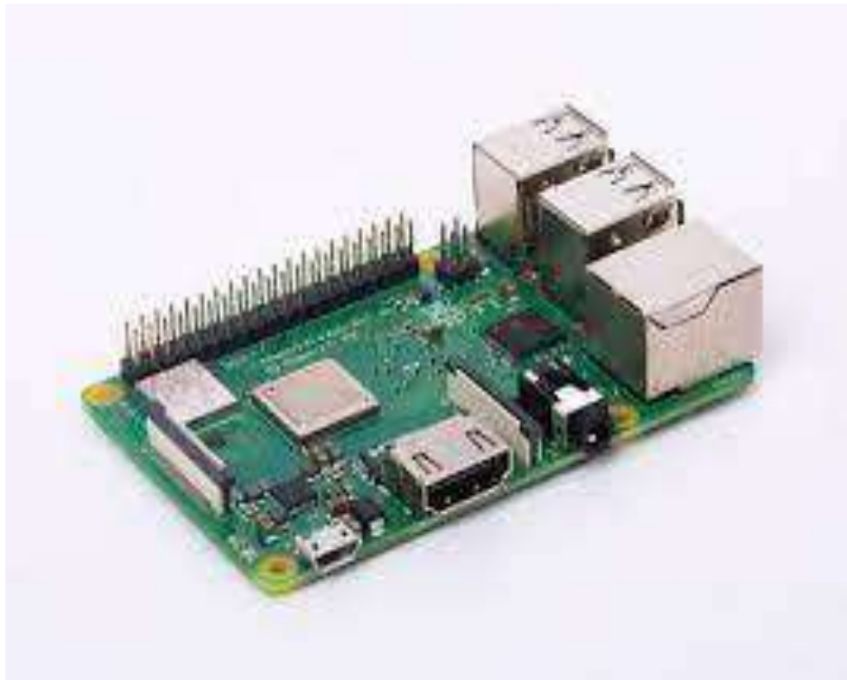
Figure 4.1: Raspberry pi 3b+ [17]
