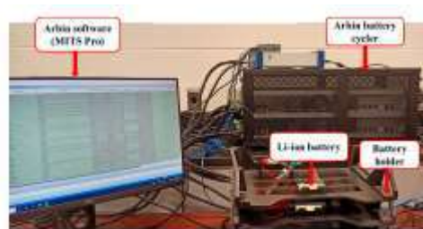
Figure 2. 24 Experimental setup for battery testing [23]
