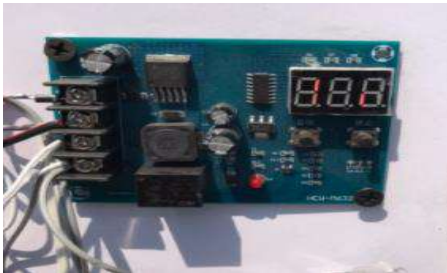
Fig 6.2 Testing of Buck converter
